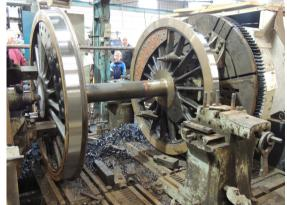
This picture shows a row of them in the workshop. The second pair from the left are for 82045, the new Class 3 tank engine being built at Bridgenorth. There were many more wheel-sets outside!
