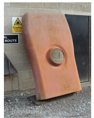
We were also shown their press that they use for shaping boiler plates, and we were told that when they set up to press a plate, they always press at least 2. A second, in case they make a mistake with the first one, but often a third which can be sold later. We saw several examples of back-heads in the yard outside, one of which is shown here.
